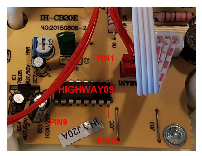
Note the LM7805 voltage regulator left to the HIGHWAY09 IC, It will be used to power HIGHWAY (Normal mode) or power the FAN constant on (Auto mode).
