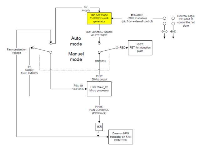
Remember: For Auto mode: Patch Power relay to Active is needed to allow power to cooker when HIGHWAY09 IC is disabled.
