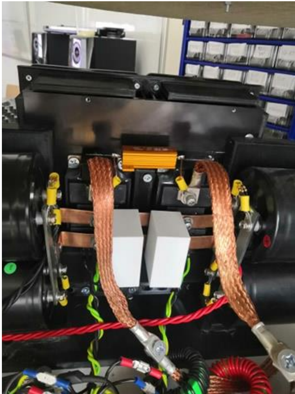
Closer look at the the inverter IGBTs on the heatsink, you can see 10kOhm power resistor for MMC charge draining and 2 Snubber capacitors (the same type i use for my MMC)
