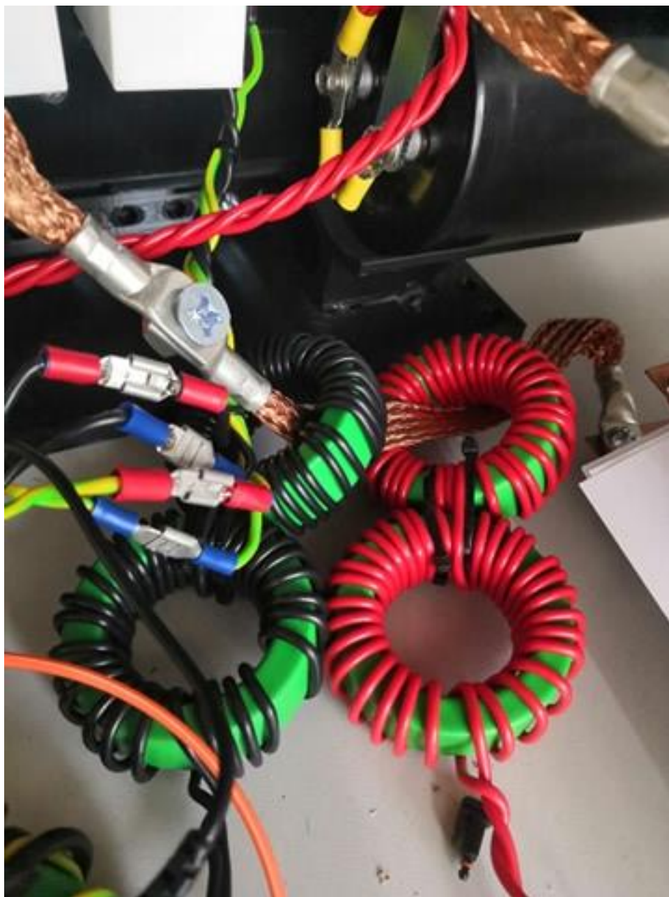
Here are the feedback (black) and OCD (red) current transformers. Cascade transformers 1:33:30 ratios.
