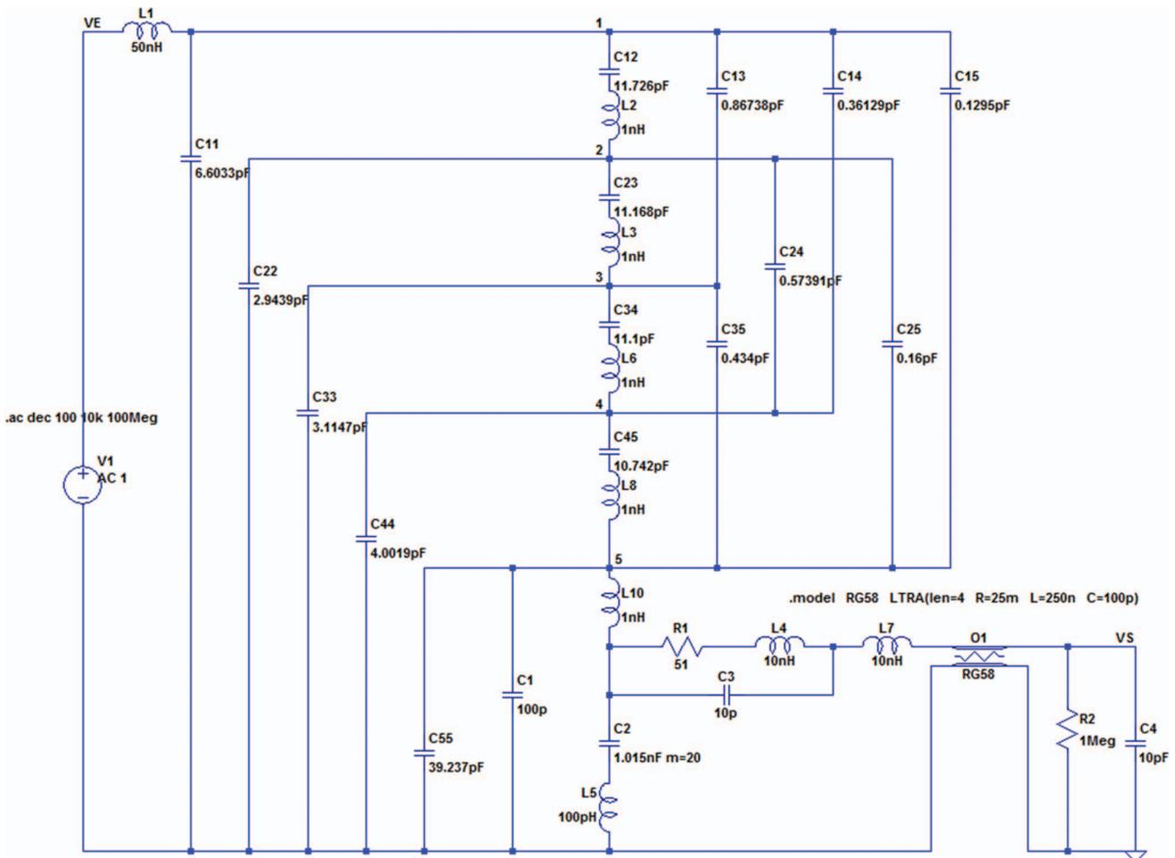
FIG. 8. (Color online) PSpice model for the Half-Megavolt probe, including the arrangement of Fig. 3.
