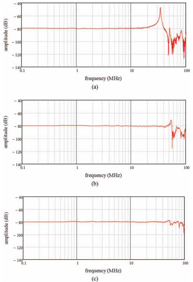
FIG. 11. (Color online) Frequency response for Half-Megavolt probe with the low-voltage arm: (a) unshielded, (b) shielded, and (c) shielded with improved electrical connections.
