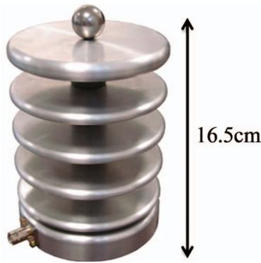
FIG. 1. (Color online) Half-Megavolt probe. The high-voltage arm is visible at the top of the assembly and the low-voltage arm is mounted on the base.
