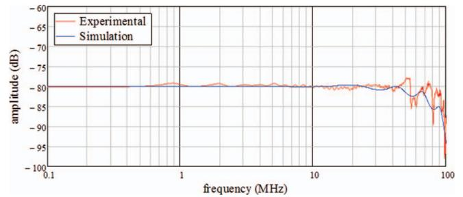
FIG. 7. (Color online) Frequency response for the Half-Megavolt probe (attenuation  $-80$  dB, i.e., 1:10 000). The corresponding theoretical prediction (smoother curve) is also shown.
