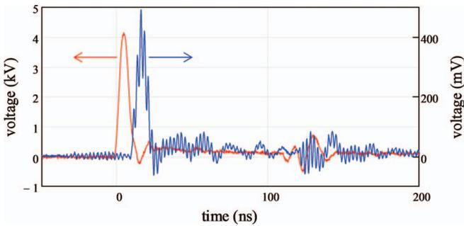
FIG. 6. (Color online) Typical signals recorded from the tests on the Half-Megavolt probe. The calibrator signals are in kV, while the probe signal is in mV, as recorded on the oscilloscope; the time origins differ mainly because of the very different coaxial cable lengths for connection to the oscilloscope.
