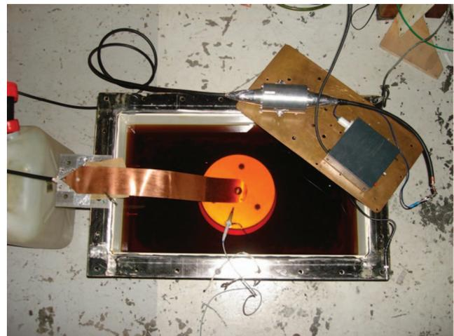
FIG. 5. (Color online) Practical arrangement for experimental determination of the frequency response of the Half-Megavolt probe.
