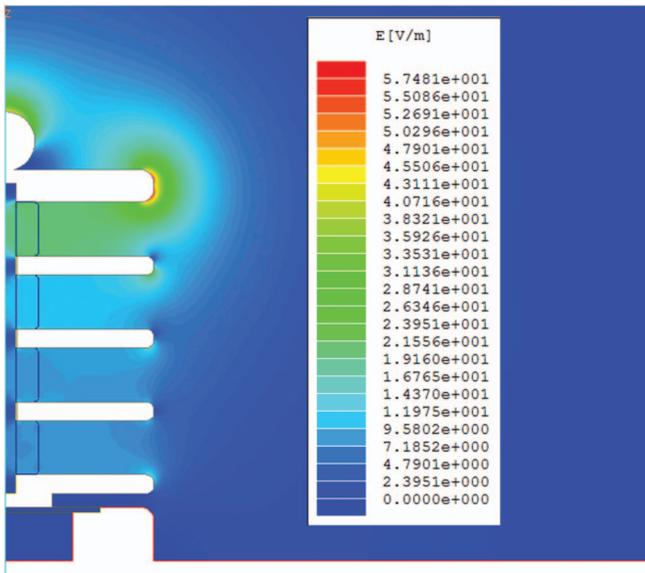
FIG. 9. (Color online) Map of electric field produced for 1 V applied on the Half-Megavolt probe. Because of symmetry only the right hand side is shown.
