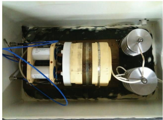
FIG. 12. (Color online) MOUNA: a compact and fully autonomous Half-Megavolt generator. The arrangement was used during the developmental tests with the assembly housed in a metallic oil-filled container. The Half-Megavolt probe is located towards the upper right corner and measures the voltage across a passive capacitive load (80 pF, located on the lower right) simulating the antenna. The load has a similar design to the high-voltage arm of the probe.
