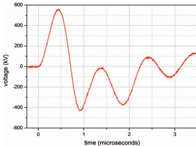
FIG. 13. (Color online) MOUNA output pulse measured by the Half-Megavolt probe during developmental tests.
