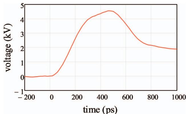
FIG. 4. (Color online) A 4 kV pulser output having a rise time of 250 ps.
