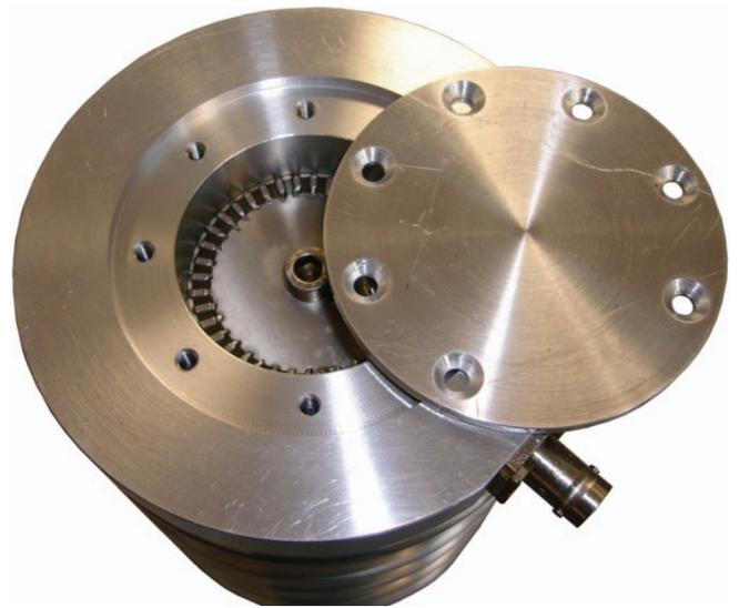
FIG. 2. (Color online) Half-Megavolt probe. The low-voltage arm is mounted at the base with the end cap of the shield opened for inspection.
