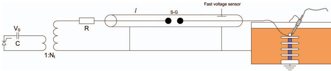
FIG. 3. (Color online) A 4 kV pulser arrangement with the voltage probe mounted inside an oil tank  $C = 470$  nF,  $V_0 = 300$  V,  $N_t = 66$ ,  $R = 1$  k $\Omega$ , and  $l = 55$  cm.
