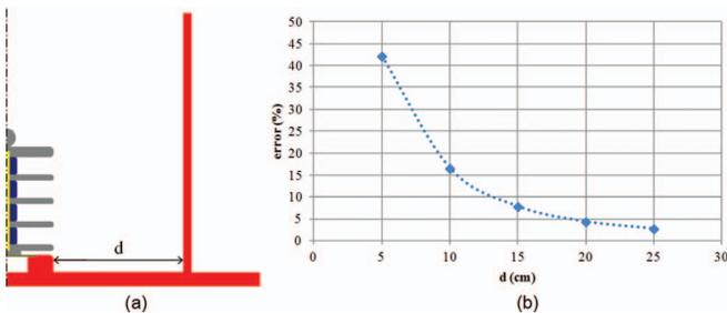
FIG. 10. (Color online) The influence of a metallic cylinder connected to ground on the probe attenuation (a) schematic indicating the distance  $d$  between the probe and the cylinder (b) estimated error introduced in the probe attenuation by the cylinder.
